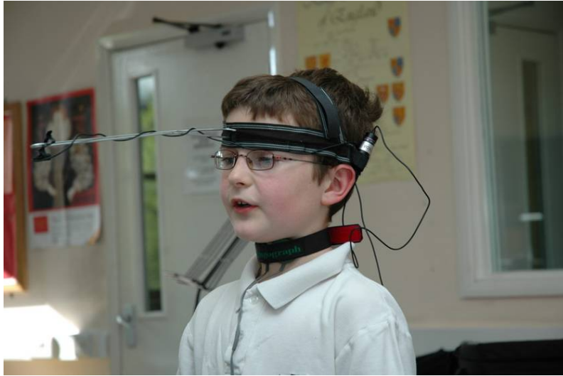
Figure 3: Boy with electrolyngograph and microphone, an illustrative example of the recording set-up (reproduced with permission)
